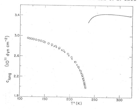
FIG. 4. Temperature dependence of  $c_{long}$  as determined from a singledomain crystal in the tetragonal ordered phase. The solid line shows the smooth-curve variation of  $c_{11}$  in the disordered phase (Ref. 4). The circles indicate data obtained on crystal Ib, and the crosses denote data obtained on the crystal with path length 2L=1.4132 cm.
